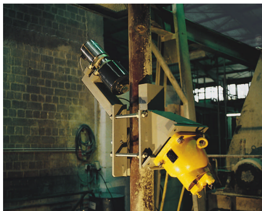
A nuclear density gauge is mounted at a 45-degree angle for small pipes or narrow measurement spans.
