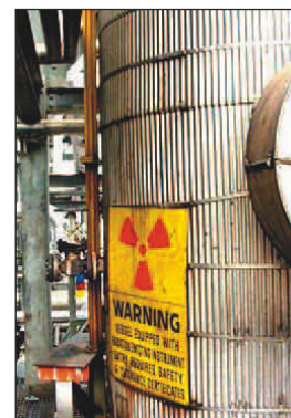
A rod-type nuclear source is mounted on the outside of a vessel.
